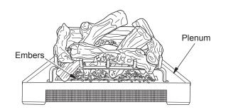
Figure 38 - Placing Ember Material on Burner
